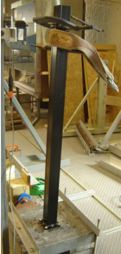
Photo No. 1 Concentrated Load at Top of a Single Post Test Setup
