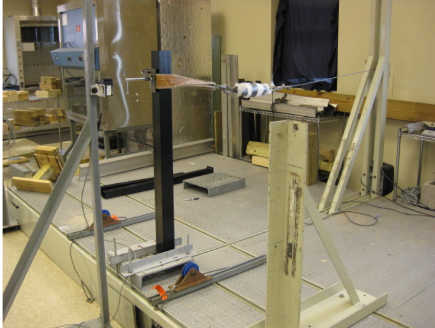
Photo No. 1 Concentrated Load at Top of a Single Post
