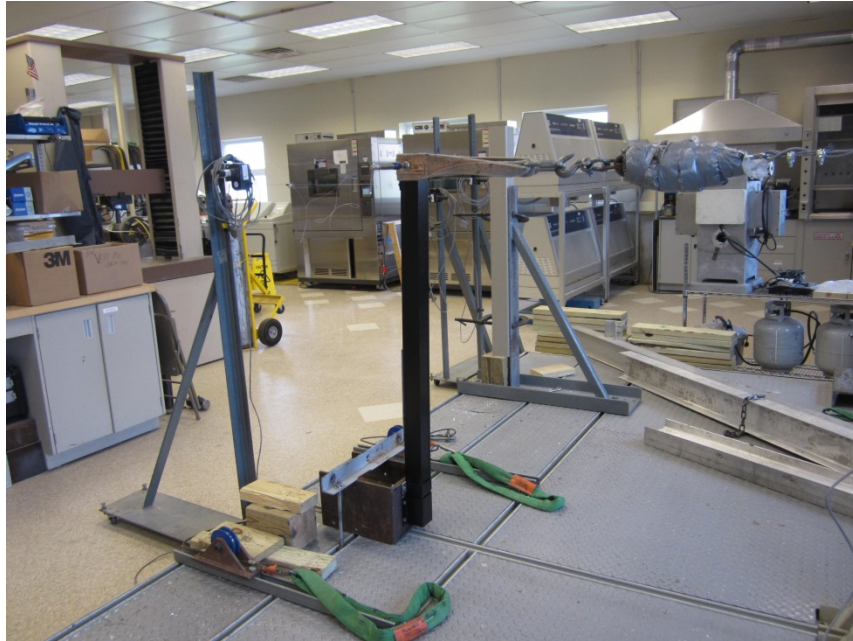
Photo No. 1 Concentrated Load at Top of Post
